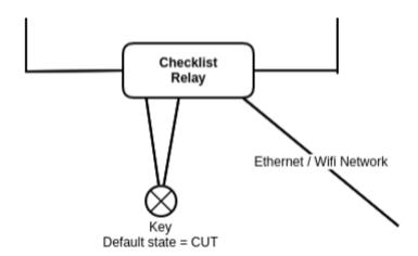
The relay in the above diagram is a PLC which provides an IP integration into the safety system which can be isolated from the existing factory network / wifi network by having the device that connects to this PLC have a back to back connection via ethernet cable. The device will be programmed to start in an open (broken) state, effectively triggering the safety relay and immobilising the machine (through the current safety mechanisms of the machine).
